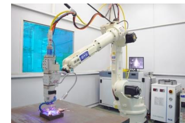
Robot hàn Fiber laser FD-V8L (Hãng OTC-DAIHEN)
