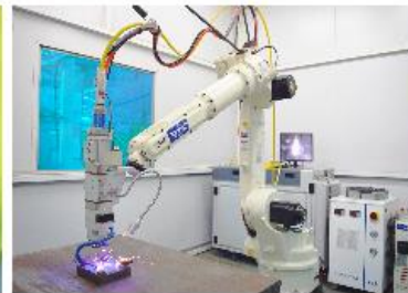
Robot hàn Fiber Laser
